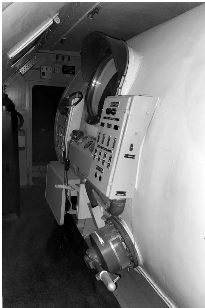
Fig. 3. PBK-70 mobile pressure chamber based on a trailer
